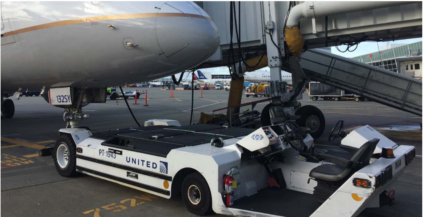
Electric LEKTRO pushback tractor pushing a United Airlines aircraft. Photo from Port of Seattle.
