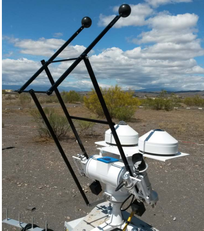
Figure 3-4. Pyrliometer, a shaded pyranometer and a shaded pyrgometer mounted on an automatic solar tracker. Photo from DLR
