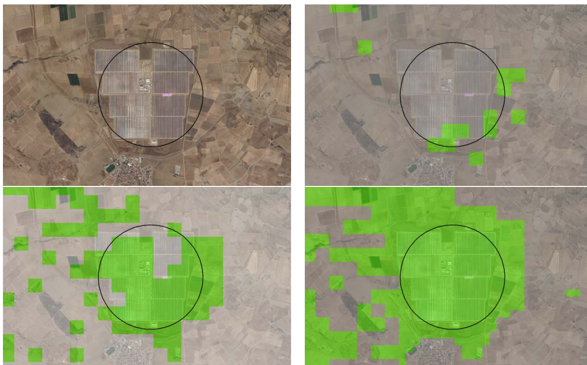
Figure 8-5. Buffer around the Orellana STE plant (Spain) and the suitable areas by the LRS1 (upper right), LRS2 (bottom left), and LRS3 (bottom right) methodologies with maximum slopes of 1%, 2%, and 3 %. Suitable zones are shown in green (Navarro et al. 2016)
