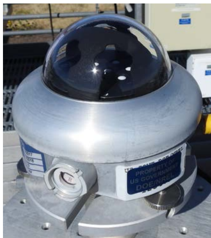
Figure 3-20. Delta-T Devices, Ltd., SPN1. Image by NREL.
