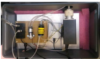
Figure 3: The Analyzer Box with (L to R) TC sensor (in a custom-built holder), pump, O_2 sensor, and valve.
