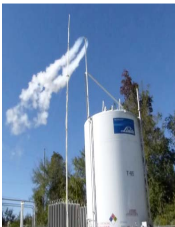
Figure 6: Deployment of the prototype Cold Hydrogen Plume Analyzer during LH 2 venting
