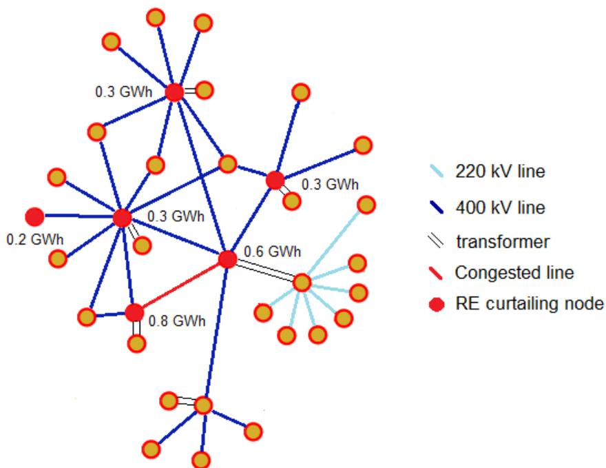
**Figure 17. Transmission map of the six Karnataka nodes that curtail RE despite flexible, intrastate thermal capacity on an example day in May**
