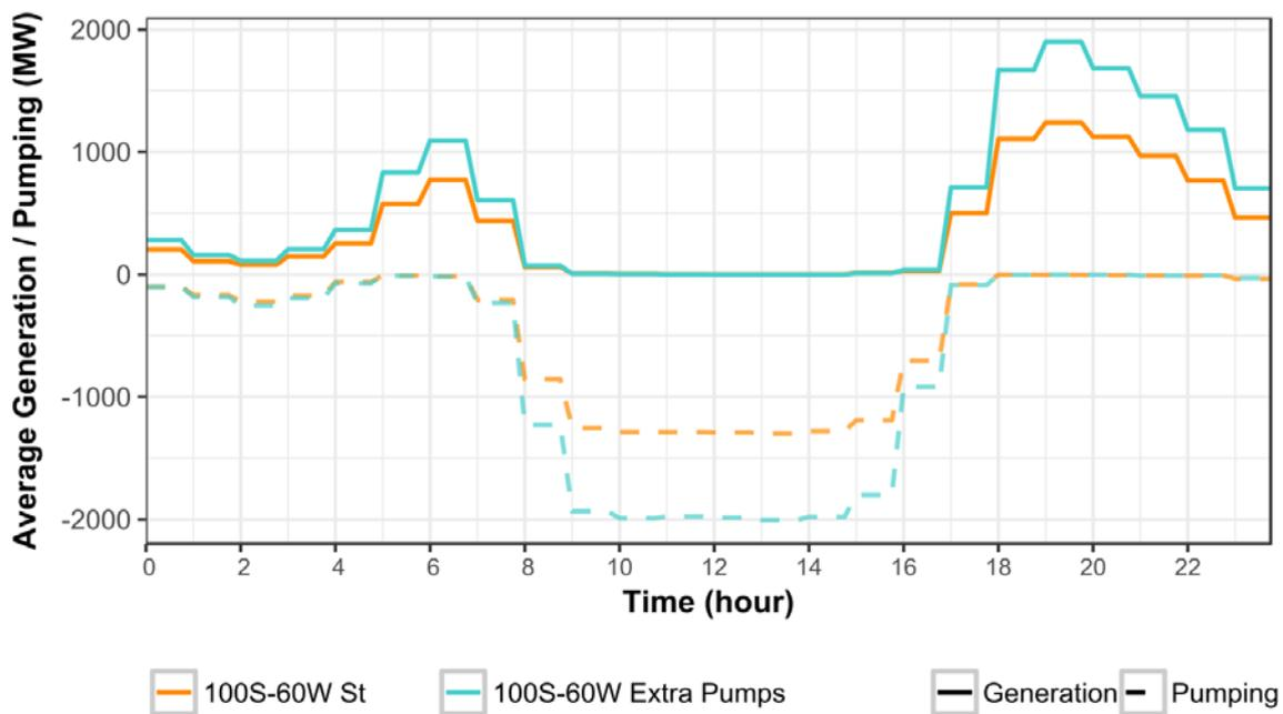
**Figure 44. Comparison of average pumping day in the Southern region with and without extra pumps**
