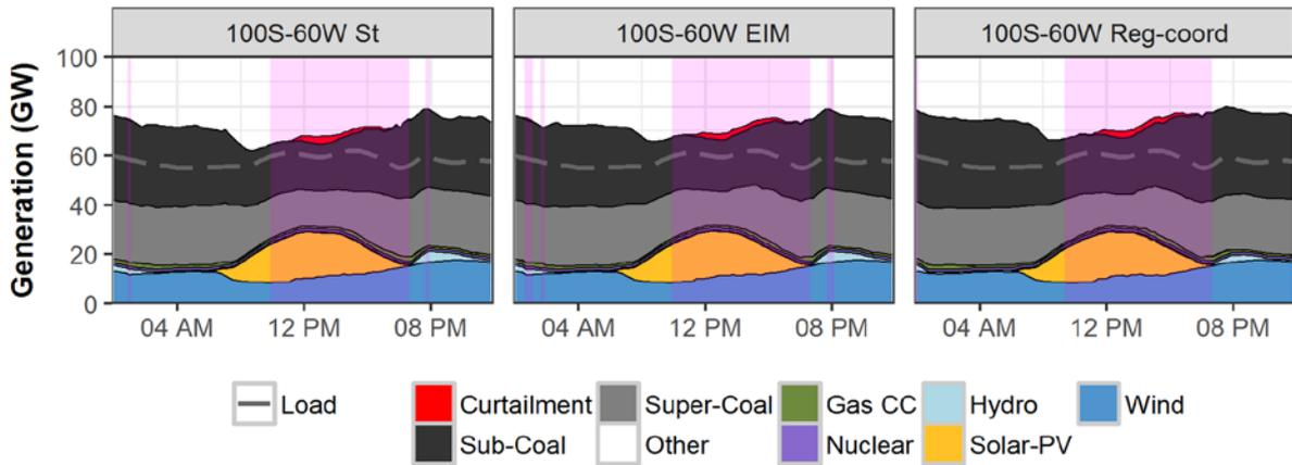
**Figure 38. Generator dispatch in the Western region on an example day in May, dispatch coordination sensitivities**
