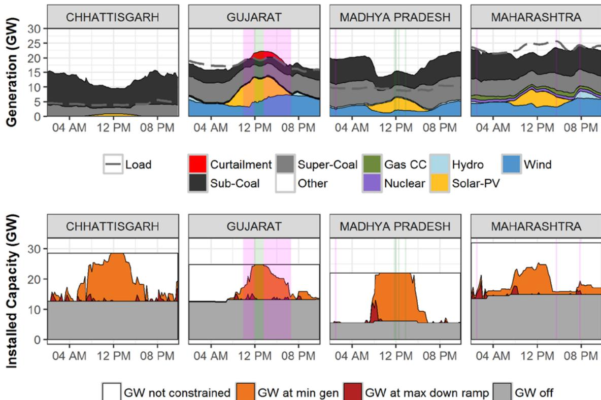
**Figure 35. Generator dispatch and thermal fleet constraints in four Western region states on an example day in May, 100S-60W**
