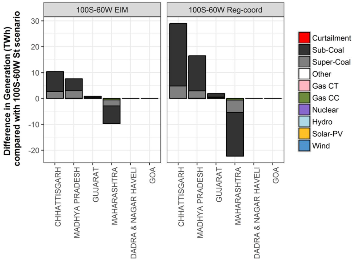
**Figure 32. Difference in generation for regional coordination compared to state dispatch, in the Western region by state**
