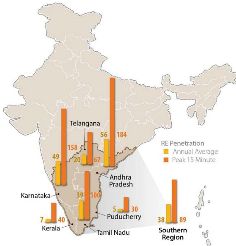
**Figure 4. Annual and 15-minute peak instantaneous penetration of RE generation as a percent of load, 100S-60W, Southern region**
