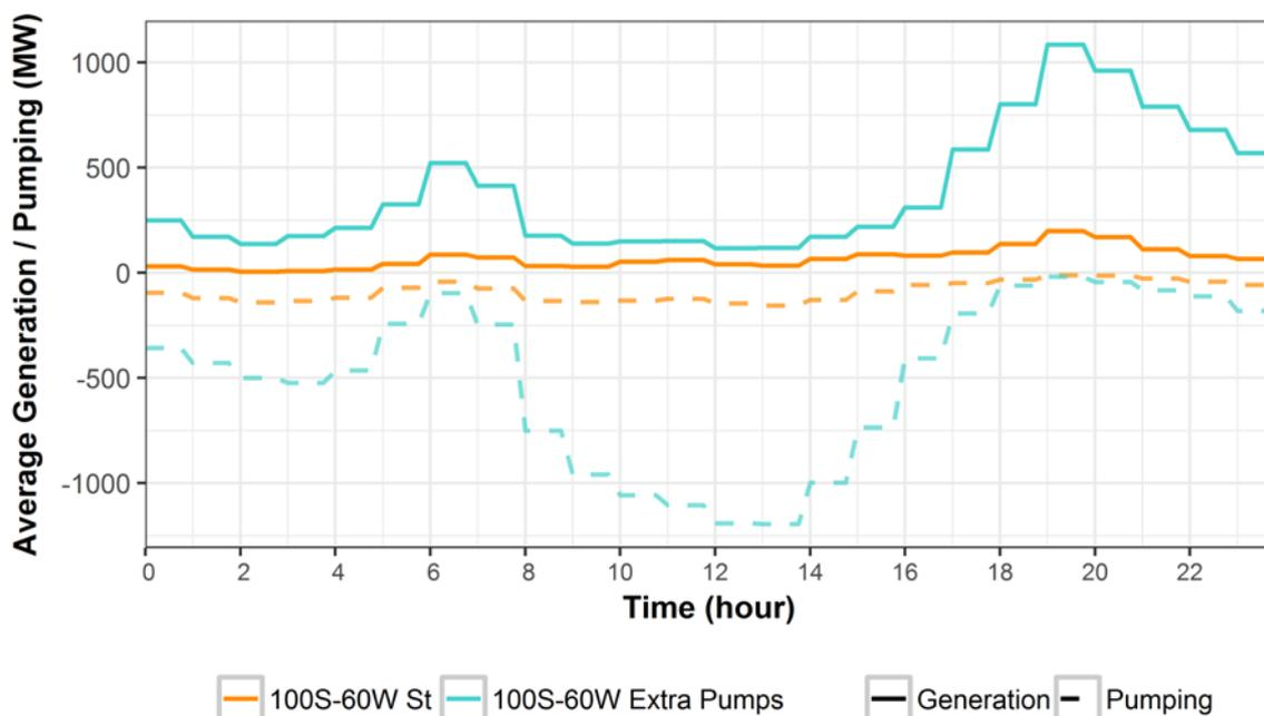
**Figure 46. Comparison of average pumping day in the Western region, with and without extra pumps**
