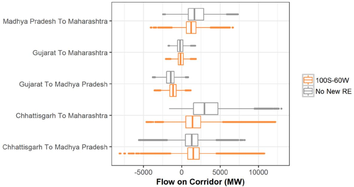
**Figure 28. Distribution of flows across state-to-state corridors within the Western region, No New RE and 100S-60W**
