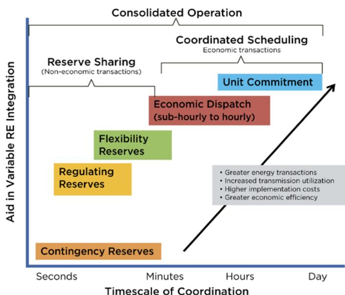
**Figure 30. When balancing areas coordinate activities over longer time scales, they are able to increase the economic benefits of coordination to support RE integration. However, coordination over longer timescales introduces greater complexity and higher implementation costs.**
