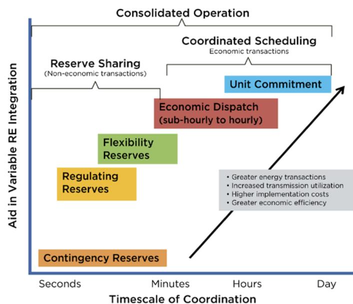
**Figure 12. When balancing areas coordinate activities over longer timescales, they are able to increase the economic benefits of coordination to support RE integration; however, coordination over longer timescales introduces greater complexity and higher implementation costs**
