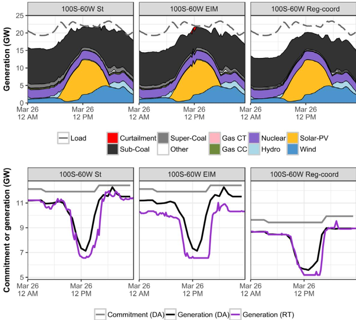
**Figure 13. Generation dispatch (top) and commitment and dispatch of coal generation (bottom) in Tamil Nadu for 26 March for state dispatch, EIM, and regional coordination**
