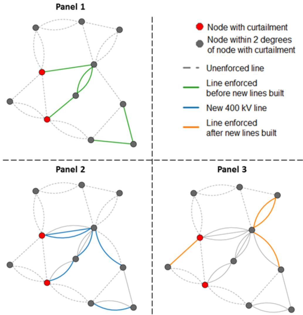
**Figure 49. Example of the iterative process of adding and enforcing lines in a small section of the Rajasthan network**
