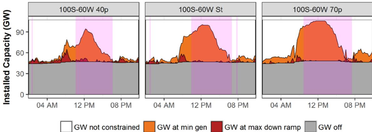
**Figure 37. Thermal fleet constraints and congestion in the Western region on an example day in May, coal flexibility sensitivities**
