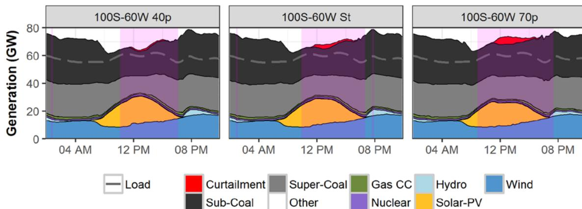
**Figure 36. Generator dispatch in the Western region on an example day in May, coal flexibility sensitivities**
