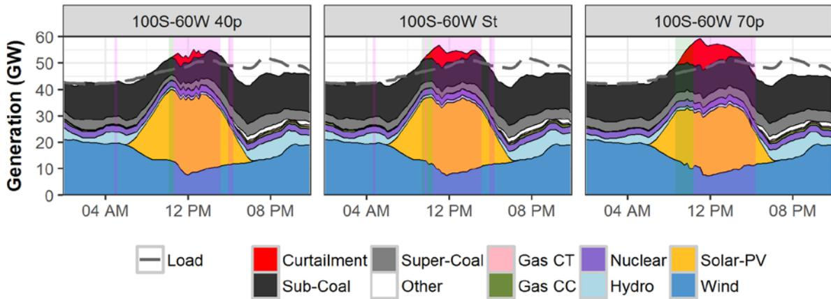
**Figure 20. Generator dispatch in the Southern region on an example day in May, coal flexibility sensitivities**
