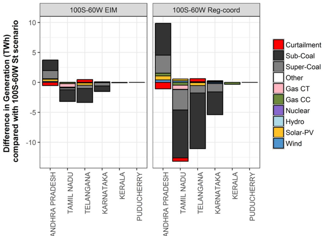
Figure 14. Difference in generation compared to state dispatch with regional coordination, in the Southern region by state
