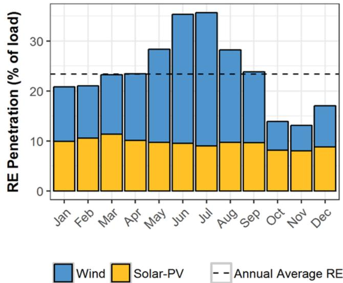
**Figure 23. Monthly wind and solar penetration as a percent of load, 100S-60W, Western region**
