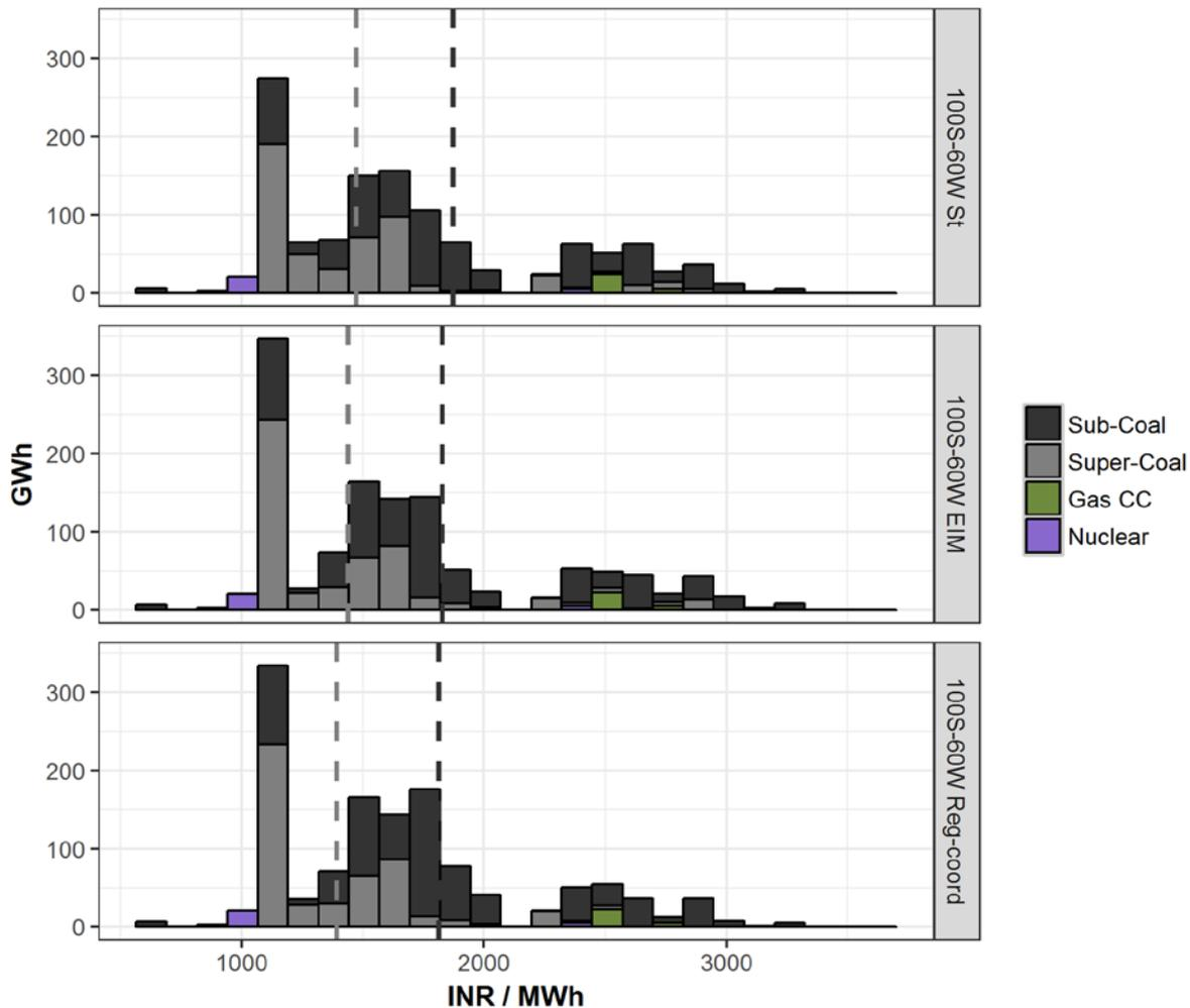
**Figure 40. Generation by variable cost band for the Western region on an example day in May across dispatch coordination scenarios**
