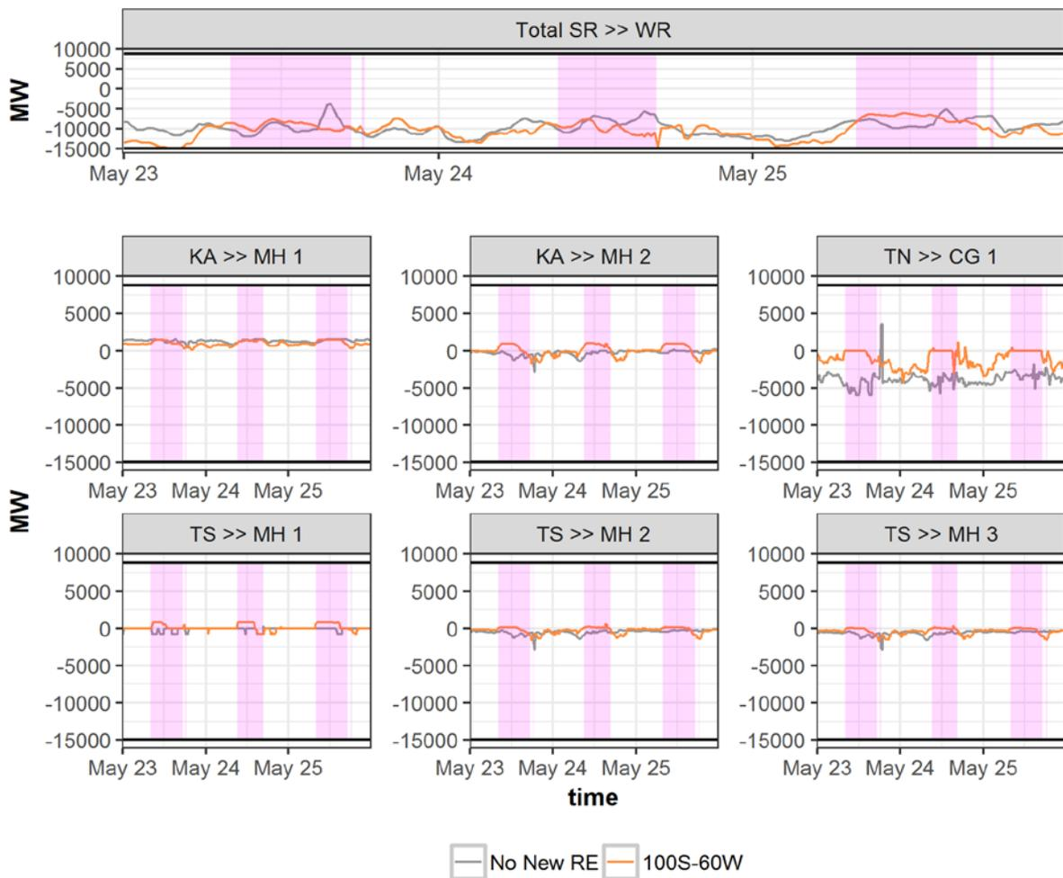
**Figure 11. Flows across SR-WR interface for a three-day period in May, No New RE and 100S-60W**
