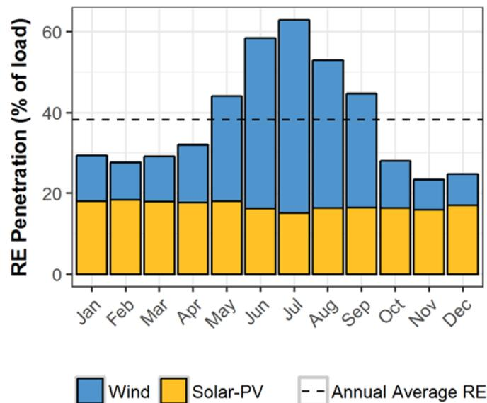
**Figure 5. Monthly wind and solar penetration as percent of load, 100S-60W, Southern region**
