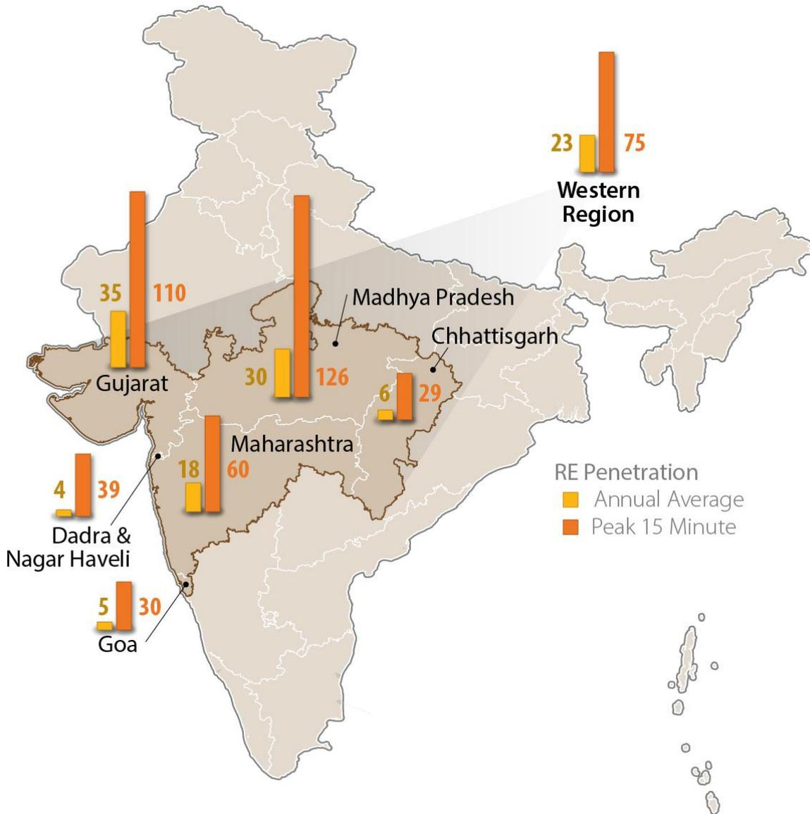
**Figure 22. Annual and 15-minute peak instantaneous penetration of RE generation as a percent of load, 100S-60W, Western region**
