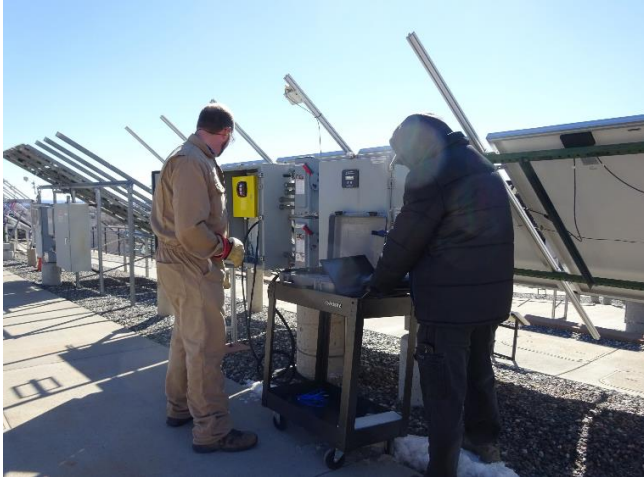
Fig. 7 Performing a periodic I-V trace test
