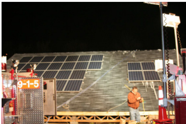
Fig. 13 UL artificial light test setup. Used with permission from UL
