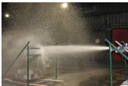
Fig. 10 UL firehose test setup – water sprayed at 1000-Vdc plate.
