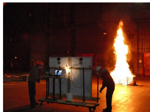
Fig. 12 UL firefight test setup. Used with permission from UL
