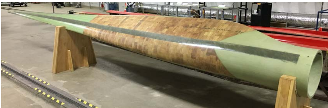
Figure 9. Nine-meter thermoplastic composite blade.
