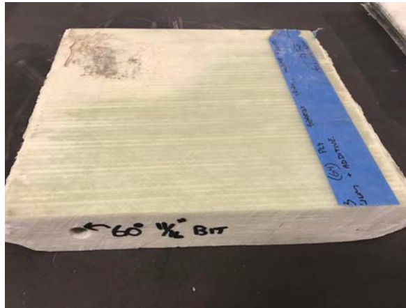
Figure 6. Hole drilled in 56-mm-thick laminate.
