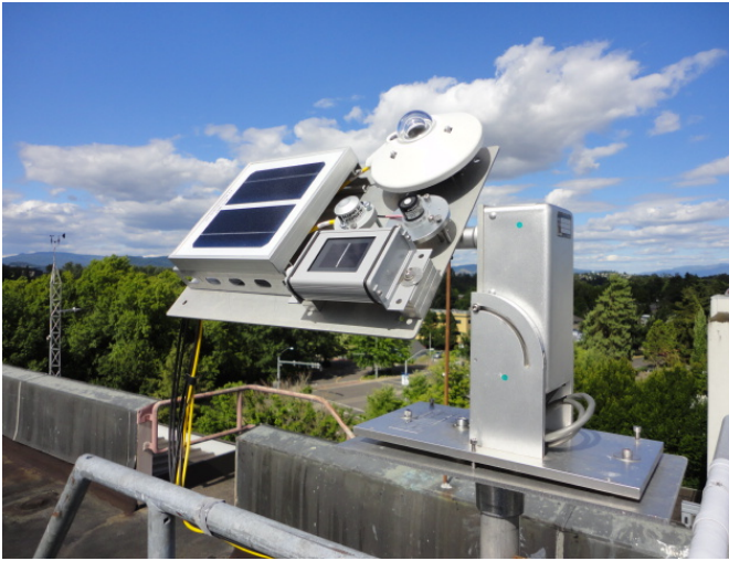
Fig. 1. One-axis tracker with sensor instruments mounted on plate at the University of Oregon station.
