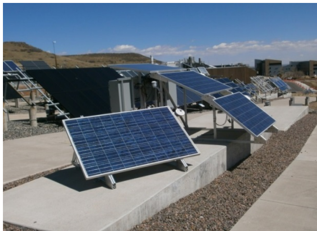
Fig. 1. PV modules with micro-inverters installed at NREL. Three PV modules are south-facing, with tilts of 10°, 25°, and 40° from the horizontal. A 4 th PV module is tilted 40° and faces 30° west of south. A 5 th PV module (not shown) is installed on a nearby two-axis tracker.
