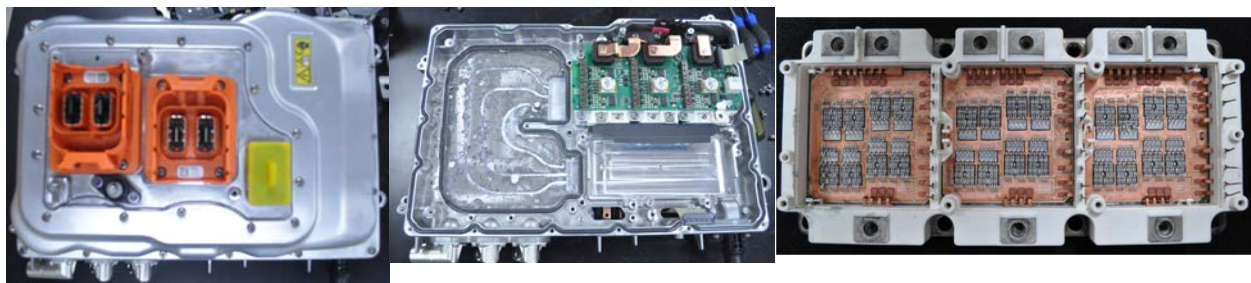
Figure I-8: Pictures of the 2015 BMW i3 inverter. The left image is the top view of the i3 EME system. The middle image shows the cold plate cooling channels. The image on the right shows the power block mounted on the cold plate.
