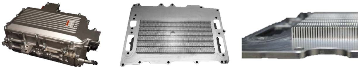
Figure I-1: Pictures of the 2014 Honda Accord inverter. The left image shows the entire power electronics system and the middle image presents the cold plate cooling channels. The image on the right shows the intricate fins directly fabricated on the cold plate.
