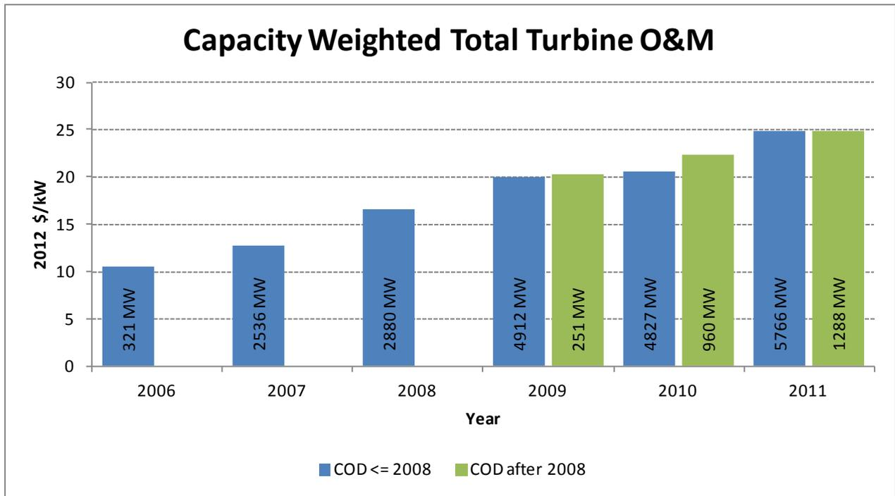
Figure 2-6. Total turbine O&M cost per kW by calendar year
