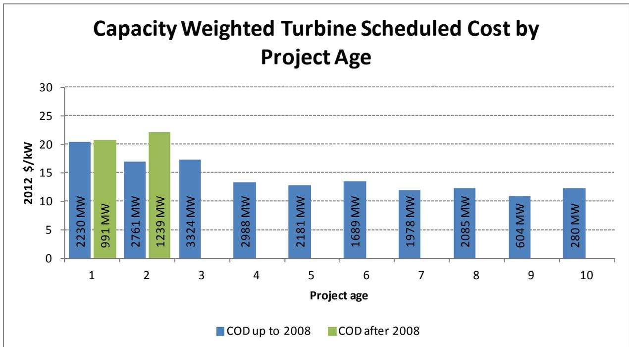
Figure 2-5. Capacity-weighted scheduled cost per kW by project age
