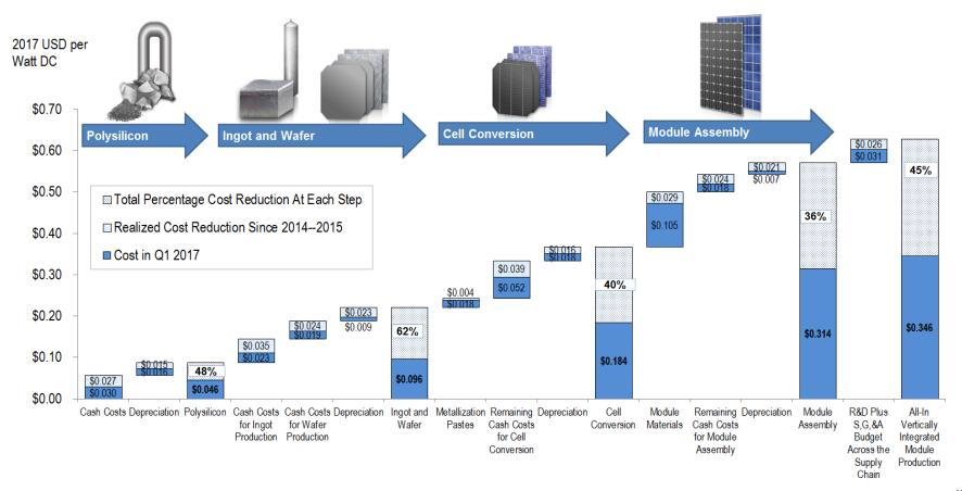
Figure 11. Updated bottom-up manufacturing cost model results for the full crystalline-silicon module supply chain from 2014/15 to Q1 2017<sup>12</sup>
