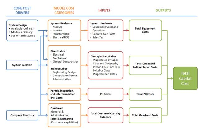
Figure 13. Residential PV: model structure
