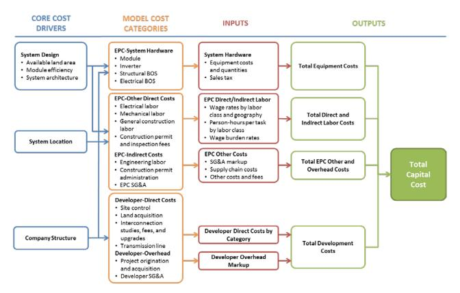
Figure 24. Utility-scale PV: model structure
