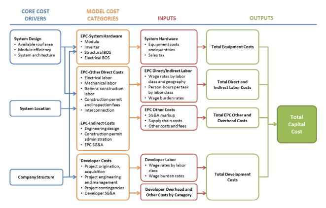
Figure 19. Commercial PV: model structure
