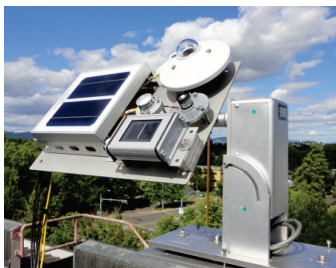
Fig. 1: One-Axis Tracker in Eugene, OR, with Kipp & Zonen CMP22, SP Lite2, LI-Cor 200A pyranometers and a RCO and an IMT reference solar cells.
