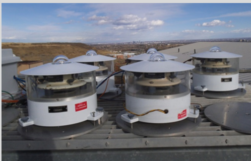
Figure 1. Test setup at NREL's SRRL consisted of five Eppley PSPs installed in Model VEN ventilators along with thermopile and housing temperature measurements. Net infrared is measured from a collocated PIR. Nighttime data were collected using two AC fans and three DC fans during January and February 2014.
