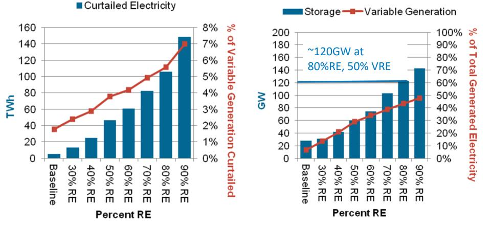
By 2050, storage capacity was estimated at 28 GW in the Low-Demand Baseline scenario, 31 GW in the 30% RE scenario, 74 GW in the 60% RE scenario, **and 142 GW in the 90% RE scenario.** Currently, there is 21 GW of pumped hydro in the Source: NREL, REF, United States.
