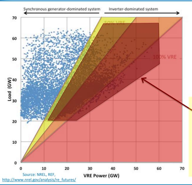
VRE vs. load for only the Electric Reliability Council of Texas (ERCOT) system at the 80% VRE transmission constrained scenario
