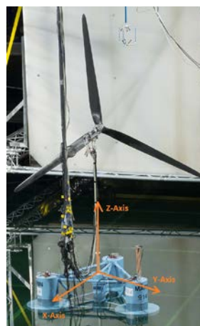
Figure 1. DeepCwind semisubmersible system as tested in MARIN's ocean basin. Positive X along downwind direction. Photo by Andy Goupee, University of Maine
