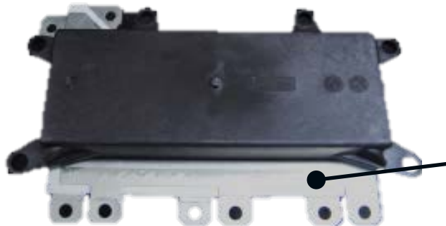
Bus bar surfaces potentially available for cooling (2015 BMW i3)
