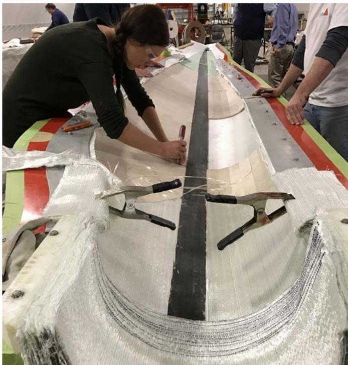
Composite manufacturing technicians work on a wind turbine blade mold at the Composites Manufacturing Education and Technology facility. The facility helps pave the way for developing innovative wind turbine components and accelerated manufacturing, while at the same time serving as a workforce development resource for a growing composite manufacturing industry. *Photo by Samantha Rooney, NREL/41767*
