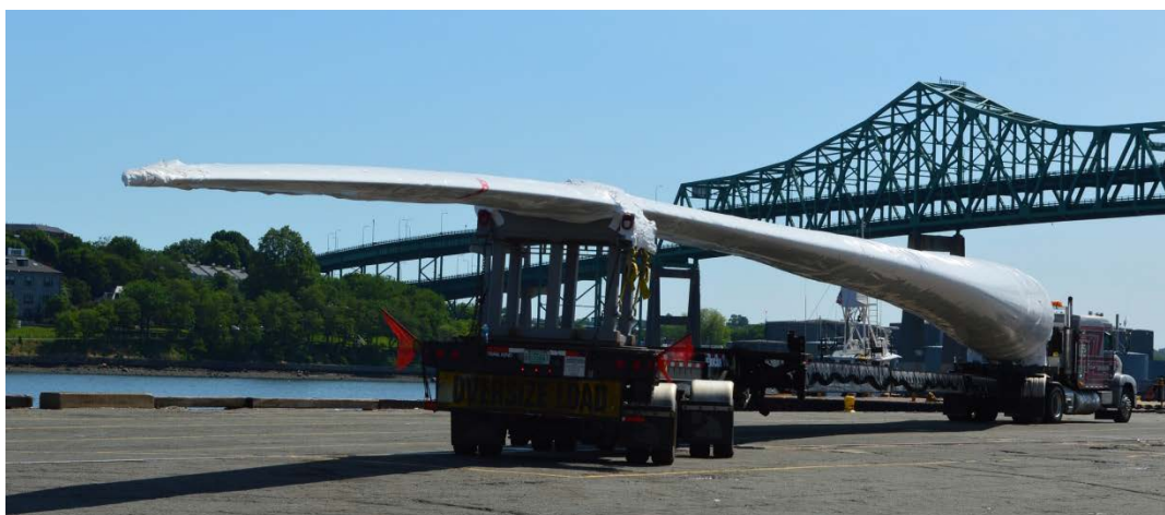
Figure 18. A turbine blade is delivered to the Wind Technology Testing Center Large Blade Test Facility in Boston. Photo from Massachusetts Clean Energy Center, Flickr
