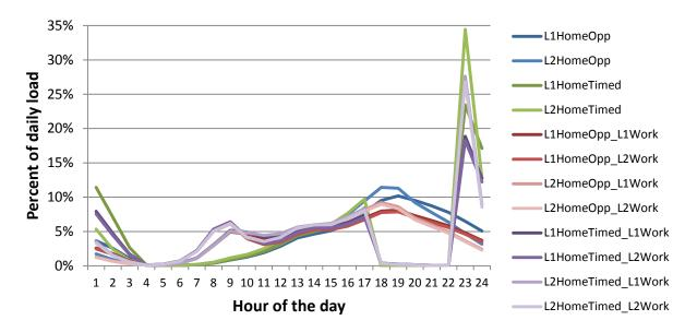
Figure 29. Charging profiles for various charger sizes and configurations
