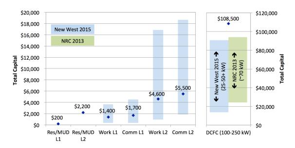
Figure ES-4. Average values used as inputs for the total capital and installation cost of EVSE by type and location in 2035
