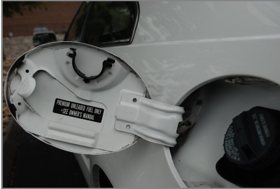
Figure 3. A typical fuel-grade guidance label inside a filler door. Photo by Scott Sluder, ORNL
