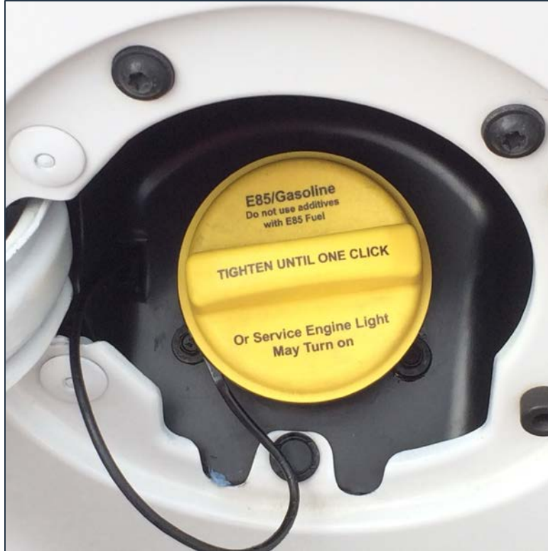
Figure 4. Yellow fill port cap on a flex-fuel vehicle. Photo by Scott Sluder, ORNL
