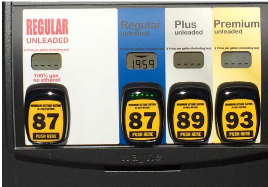
Figure 1. Anti-knock index (AKI) labels on a typical fuel dispenser. Photo by Scott Sluder, ORNL
