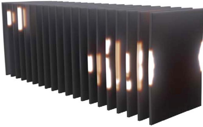
Figure 5: Blender rendered exploded view of the in-plane current density distribution on the surface of the active anode and cathode, illustrating the locations of the short circuit.
