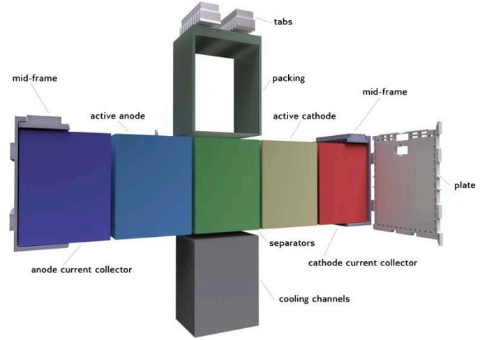
Figure 2: 3D expanded view of several of the battery module's layers and components.
