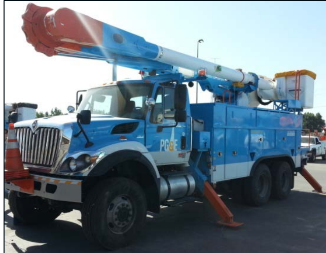
Figure 2. Altec AM material handler double-bucket truck
