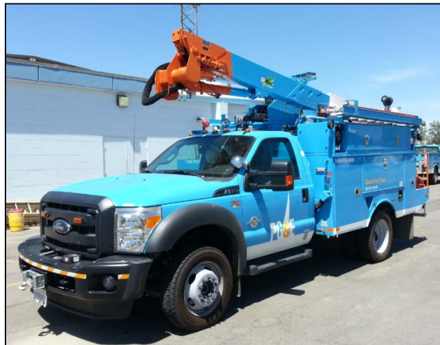
Figure 1. Altec AT trouble bucket truck
