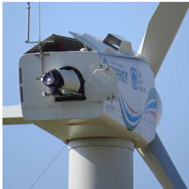
Figure 4: The DTU SpinnerLidar installed on the SWiFT turbine. Photo by Tommy Herges, Sandia.
