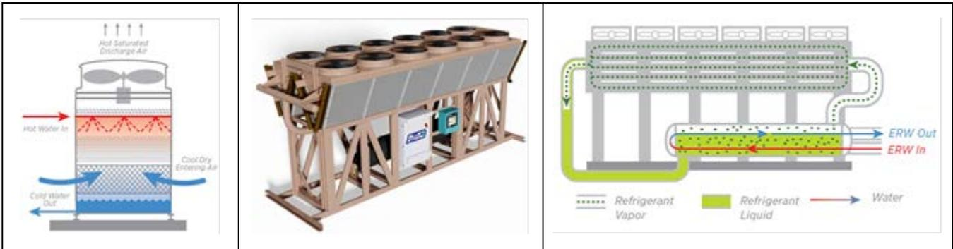
**Figure 1** (a) Counterflow cooling tower diagram, (b) TSC, and (c) conceptual design of the TSC.
