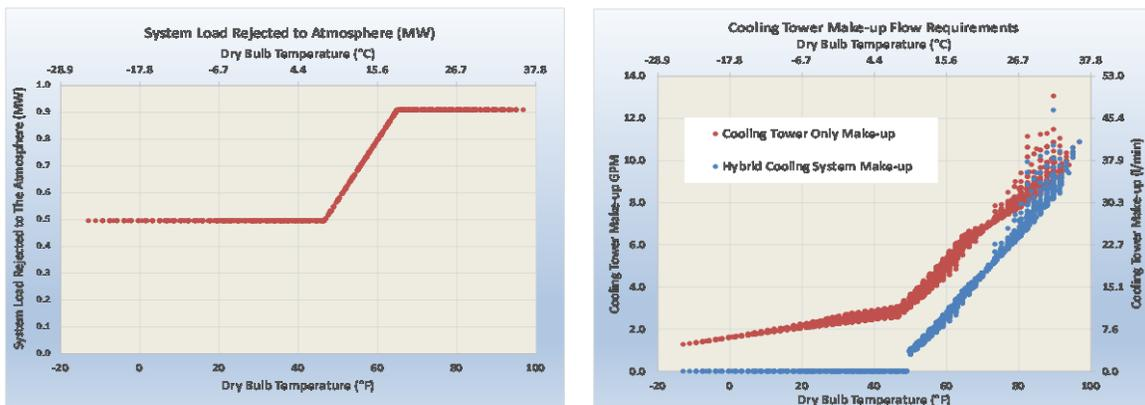
Figure 5 (a) System load rejected to the atmosphere and (b) cooling tower make-up flow rate.
