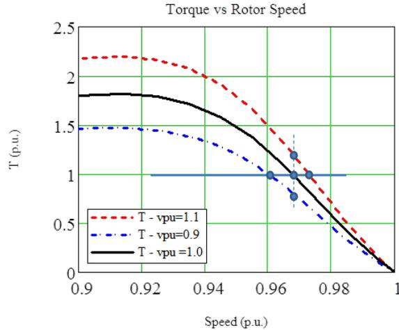
**Figure 2. Torque-speed characteristic of an induction motor under varying voltage magnitudes**
