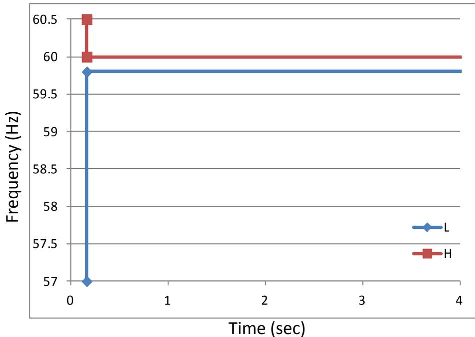
**Figure 8. Representation of frequency versus maximum clearing time as described in IEEE 1547 [12]. H = upper frequency limit, L = lower frequency limit.**
