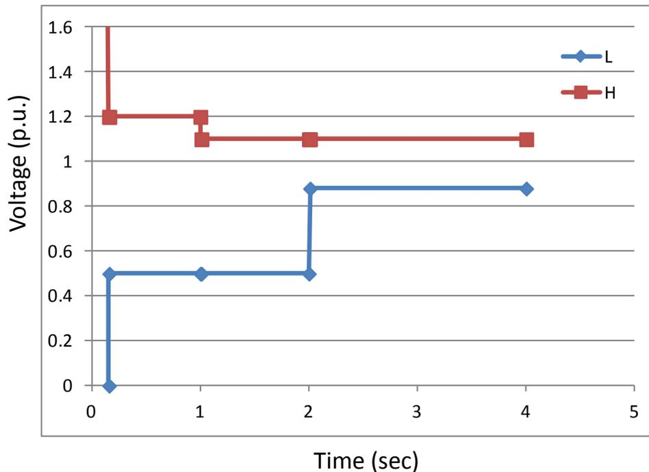
**Figure 5. Representation of voltage versus maximum clearing time as described in IEEE 1547 [12]**
