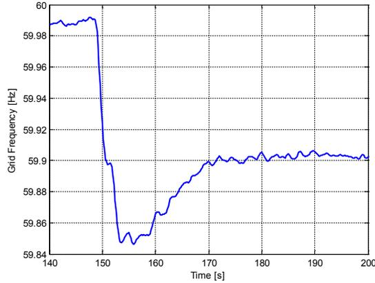
**Figure 7. An example of frequency dip caused by a loss of generation—recorded at the National Wind Technology Center of the National Renewable Energy Laboratory**
