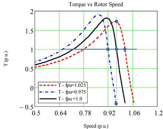
**Figure 6. Torque-speed characteristic of an induction motor under varying frequency**
