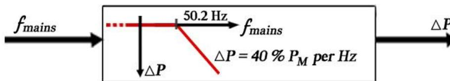
**Figure 4. Active power output during underfrequency/overfrequency conditions [1]**
