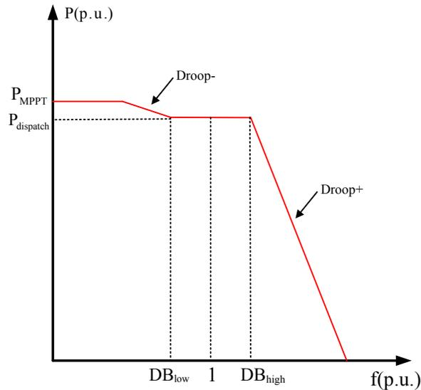
**Figure 3. Variable droop characteristic curve of active power versus frequency for PV**
