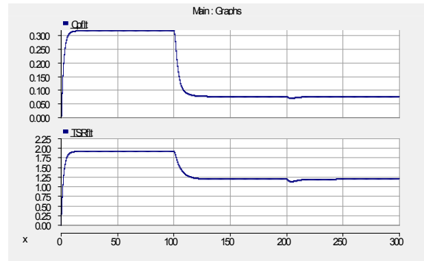
Fig. 6. Operating C_p and the TSR as the water flow changes in an unstable operation
