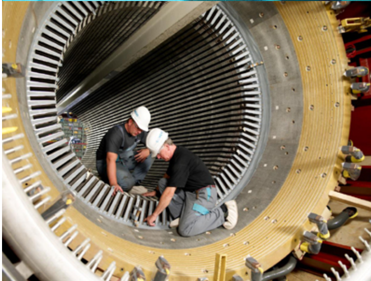
Generator Sgen 4,000-W (Siemens) 1,300–2,235 MVA
