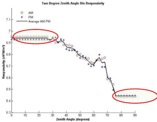
**Figure 2:** Example of responsivity as a function of SZA for Eppley Laboratory, Inc.’s Standard Precision
