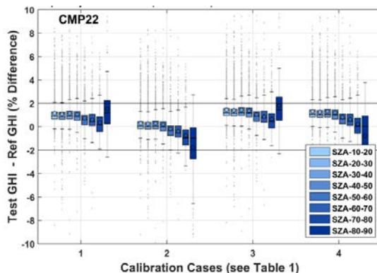
**Figure 1:** Indoor and outdoor calibration comparison of the reference GHI irradiance to the CMP22 test radiometer irradiance.
