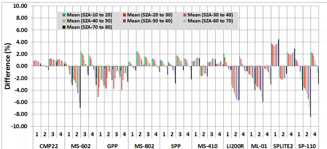
**Figure 3:** Mean percent differences for six thermopile pyranometers (first six) and four photodiode pyranometers (last four).
