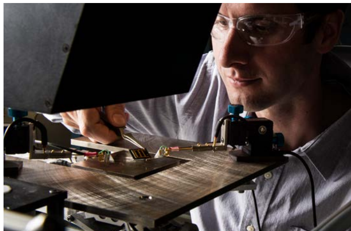
NREL researcher positions a 4-junction inverted metamorphic solar cell on a THIPSS flash simulator for measurement under concentrated light. Photo by Dennis Schroeder, NREL 32509
