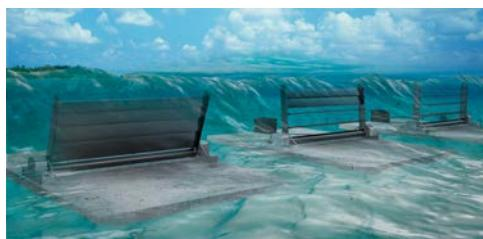
*NREL's "Wave Energy Conversion Devices with Actuated Geometry" record of invention features individually controlled flaps that open and close depending on wave conditions. This results in improved energy capture without overloading the generator and could cut the cost of wave energy in half.* Illustration by Joshua Bauer, NREL.
