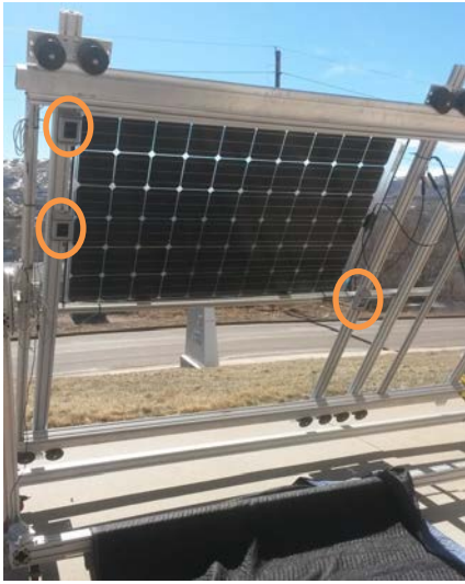
Fig. 8: Outdoor bifacial module measurement configuration, showing three rear-facing reference cells (circled) and dark ground cover to reduce the G_{rear} gradient.
