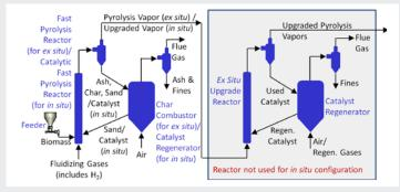
Conceptual design of *in situ* and *ex situ* catalytic fast pyrolysis processes as detailed in NREL/TP-5100-62455.
