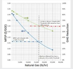
Analysis showing the tradeoff between production cost (MFSP) and greenhouse gas reduction with the use of supplemental natural gas in a biomass conversion process as shown in NREL/ TP-5100-62402.
