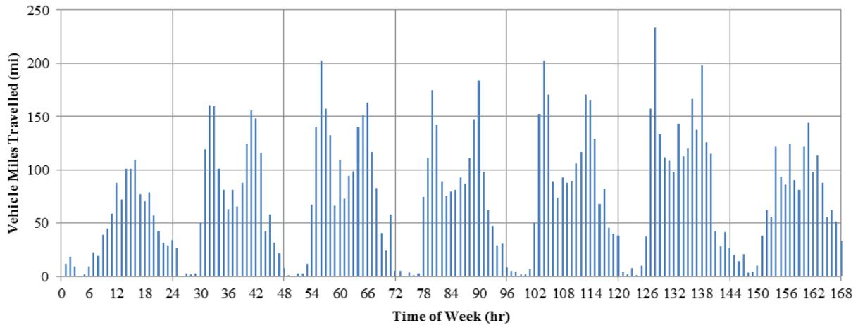
Figure 1: Hourly distribution of VMT on selected roadways for a "typical" week of travel
