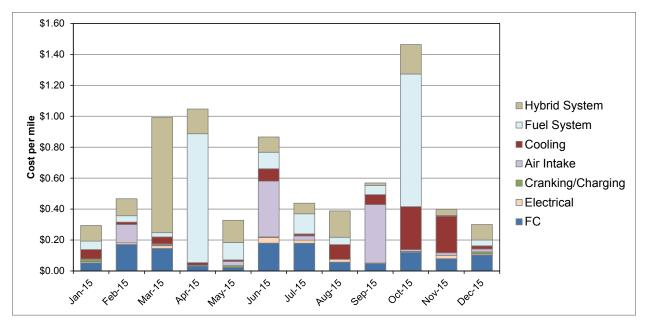
Figure D-3. Monthly propulsion system cost per mile by sub-category for the ZEBA buses
