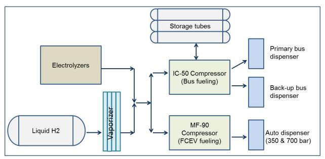
Figure 6. Block diagram of the Emeryville station
