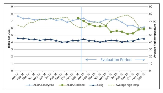
Figure 19. Average fuel economy for the fuel cell and diesel buses (evaluation period)
