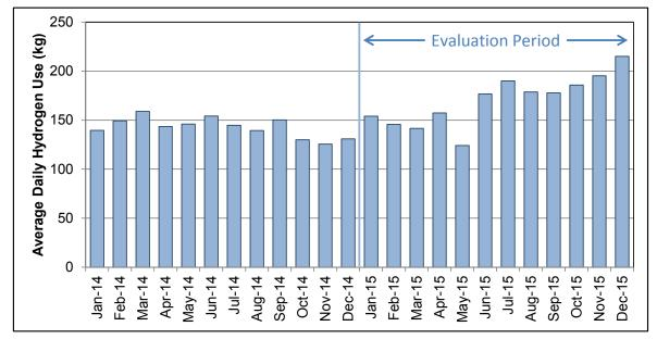
Figure 10. Average hydrogen dispensed per day at AC Transit's hydrogen stations (excluding 0 kg days)
