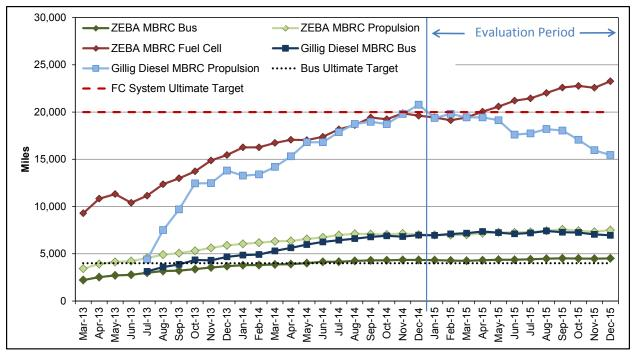
Figure 20. Cumulative MBRC for the FCEBs and diesel buses
