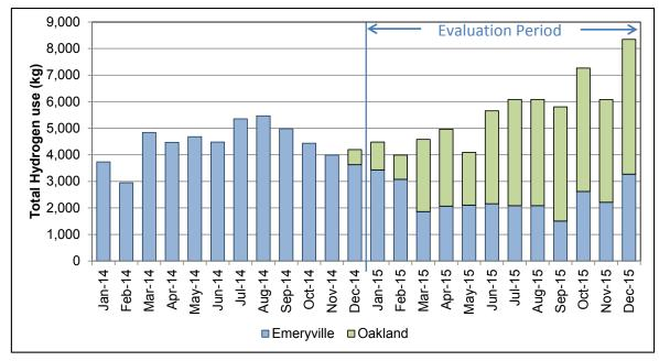
Figure 11. Total hydrogen dispensed per month at AC Transit's hydrogen stations
