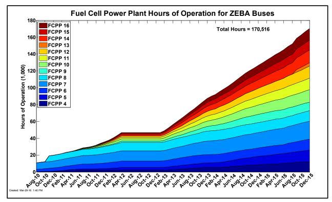
Figure 13. Cumulative FCPP hours on the ZEBA buses
