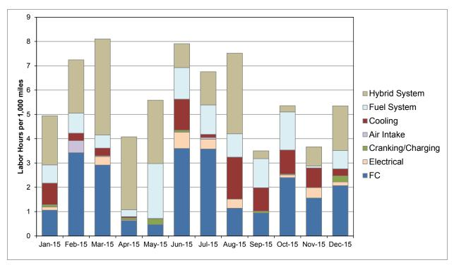
Figure D-2. Monthly propulsion system labor hours by sub-category for the ZEBA buses
