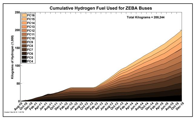
Figure 12. Cumulative hydrogen dispensed into the buses through December 2015<sup>9</sup>
