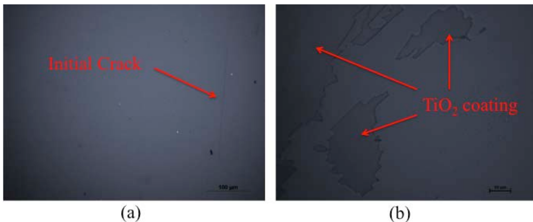
Figure 5: (a) Surface morphology of unaged TiO 2 /PET system, (b) Surface morphology of UV aged TiO 2 /PET system after adhesion test.
