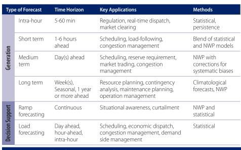
Various types of VRE forecasting have different time horizons, methods, and applications in system operations [2].
