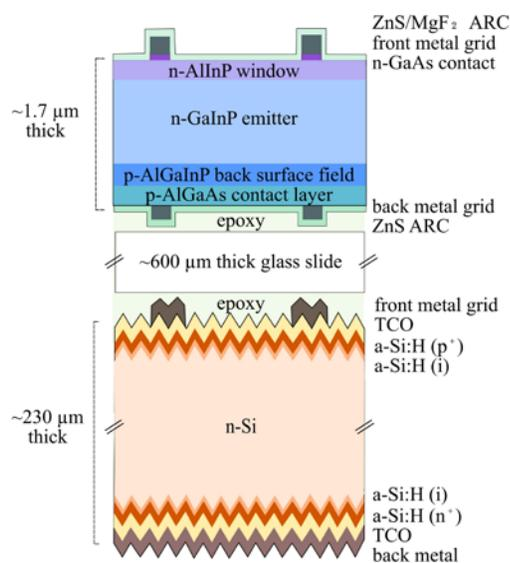
*Schematic cross-section showing NREL's GaInP top subcell and CSEM's Si bottom subcell epoxied onto an intervening glass slide to form the completed mechanically stacked dual-junction device.* Illustration by Stephanie Essig, NREL
