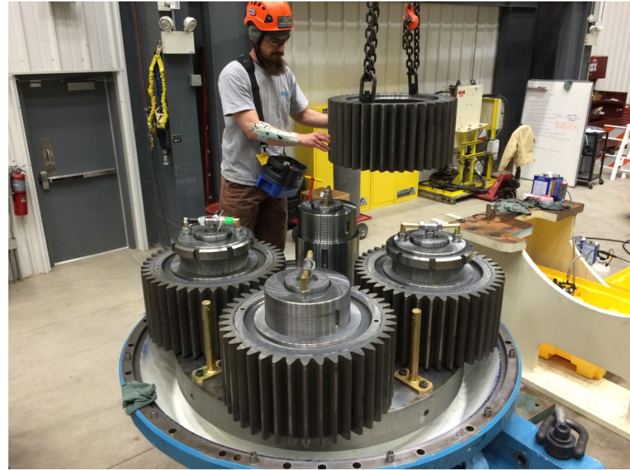
NGD gearbox planetary section. Photos by Chris Halse, NREL 33353 and Jon Keller, NREL 33341
