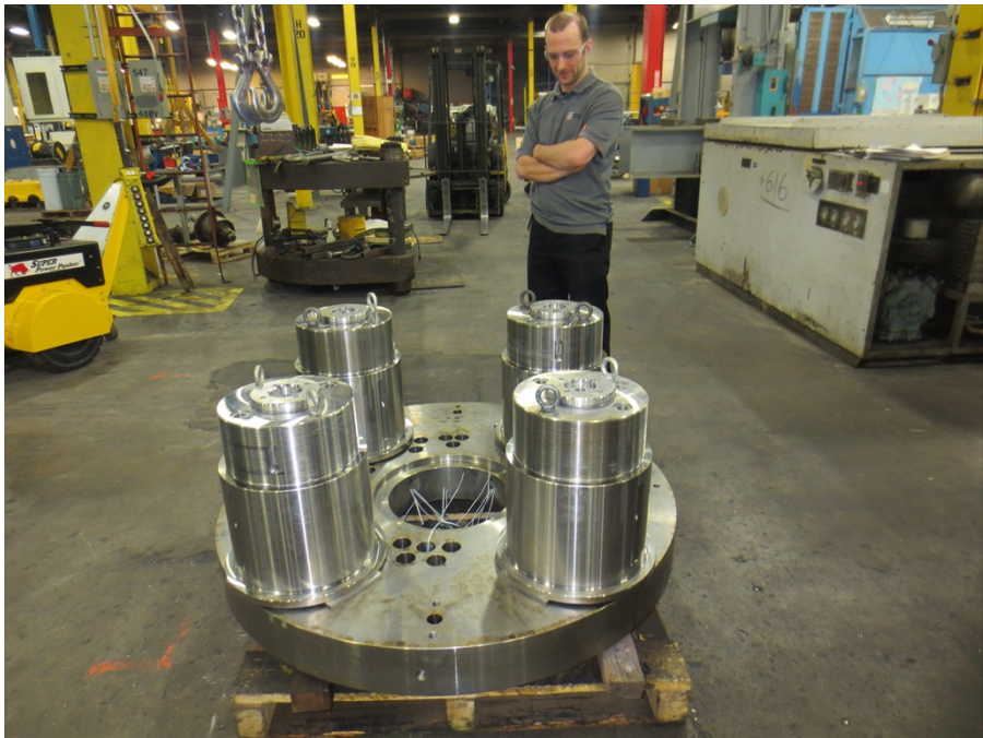
NGD gearbox planetary section. Photos by Chris Halse, NREL 33353 and Jon Keller, NREL 33341
