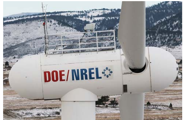
Figure 3: The Avent 5-Beam installed on the nacelle of the CART2 at the NWTC. (Photo Credit: Lee Jay Fingersh, NREL 33621)
