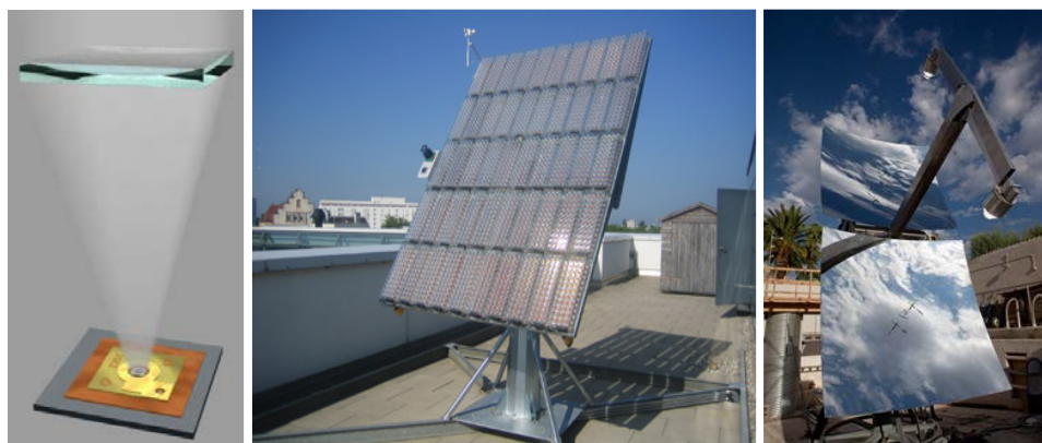
Figure 1: Left and middle: Example of a CPV system using Fresnel lenses to concentrate the sunlight: FLATCON ® concept originally developed at Fraunhofer ISE. Right: Example of a mirror-based system developed by the University of Arizona, USA [6].
