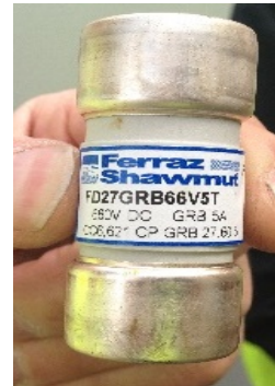
Figure 2. A 5-amp ground fault fuse
