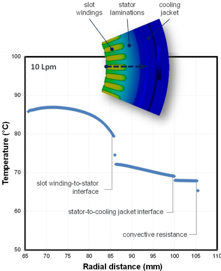
Figure I-6: Temperature profile through the motor stator depicting the thermal path from the inner surface of the slot liner to the coolant. The arrow in the upper image indicates the thermal path.
