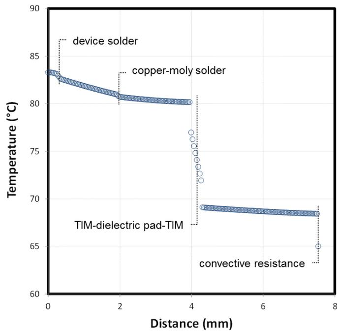
Figure I-11: Temperature profile through the inverter depicting the thermal path from the IGBT to the coolant. The TIM-dielectric pad-TIM layers constitute a significant thermal resistance to the power modules.
