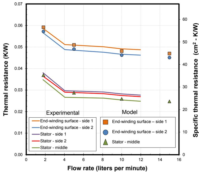
Figure I-3: Experimentally measured and model-predicted thermal resistance values for different parts of the 2012 Nissan LEAF motor stator. Note: Side 1 refers to the end-winding side of the motor that has the electrical connections.
