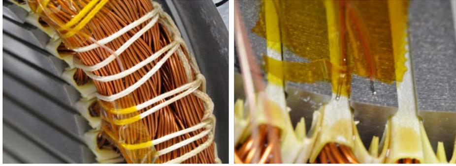
**Figure I-2: Pictures show the thermocouple placements on the end-windings (left) and stator surfaces (right).**
