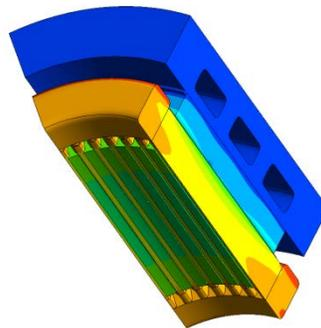
Figure I-5: FEA-generated temperature contours of a one-eighth model of the motor stator.
