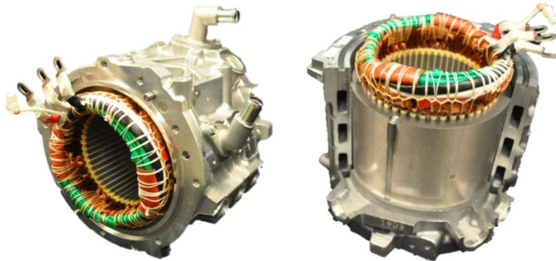
Figure I-1: Pictures of the 2012 Nissan LEAF motor. Image on the right shows the cooling jacket sectioned-off to reveal the internal coolant channels.
