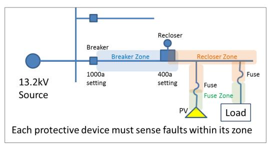
Figure 2.10. PV may desensitize protection devices to faults
