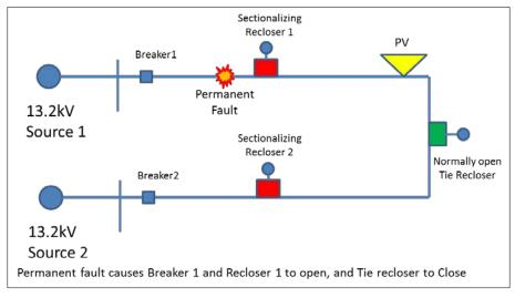
Figure 2.19. Reconfiguration in the presence of PV
