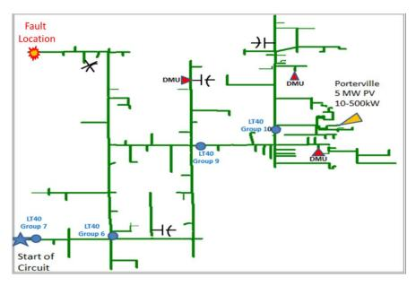
Figure 3.19. Porterville example study results-detailed fault assessment of the circuit
