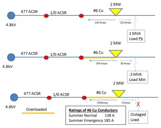
Figure 2.21. Overload during normal and contingency conditions
