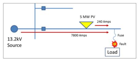
Figure 2.8. Impact of PV on fuse interruption ratings
