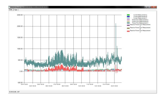
The tabular format provides sorting capabilities to quickly find erroneous high, low, or missing data. The time plot format allows for the rapid visualization of changes and also shows missing data. (See the figure below.)
