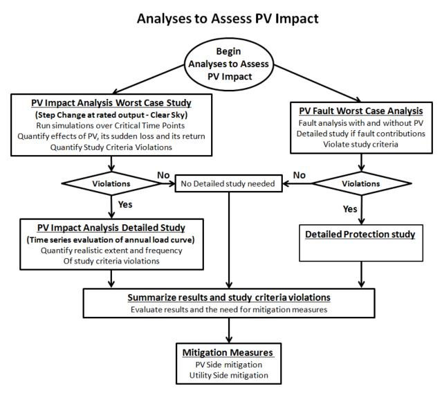
Figure 3.2. Flowchart for performing PV impact studies
