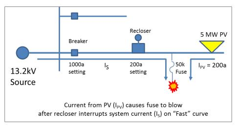
Figure 2.13. Illustration of nuisance fuse-blowing caused by large PV penetration
