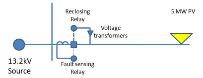
The PV must disconnect prior to the first reclosing Voltage sensing can block reclosing for additional security
