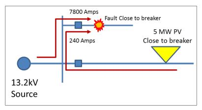
Figure 2.9. Impact of PV on breaker interruption ratings
