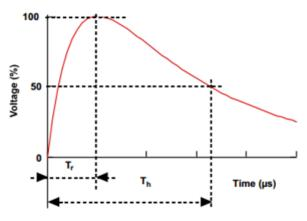
Figure 2.6. Example of transient overvoltage
