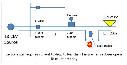
Figure 2.15. Illustration of sectionalizer miscount because of PV
