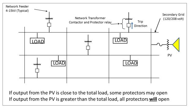
Figure 2.16. Reverse power relay operation because of PV
