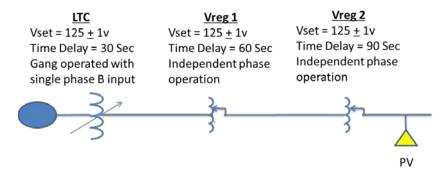
Figure 3.4. Example of voltage regulators and control details
