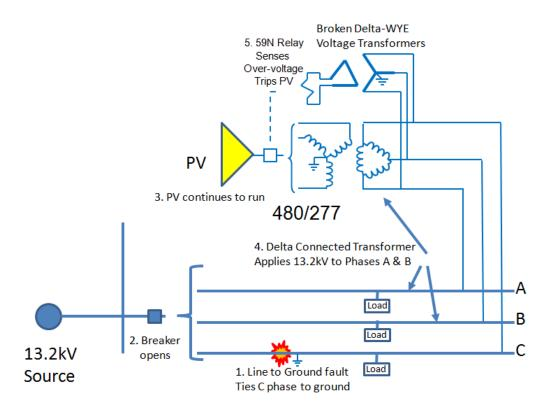
Figure 2.12. PV may cause line-to-ground overvoltage
