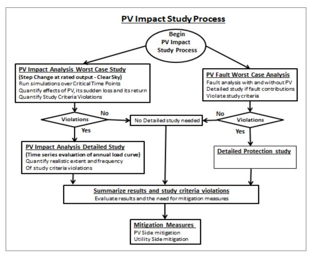
Figure 3.8. PV impact study flowchart
