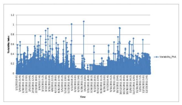
Figure 3.17. Porterville example study results—5-MW PV site radiant variability analysis by minute
