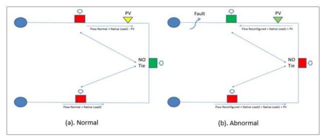
Figure 2.20. (a) Normal and (b) abnormal configuration of an auto loop system, red indicates a closed switch, green indicates an open switch
