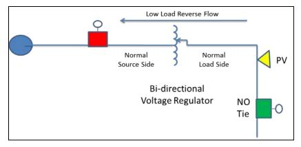
Figure 2.7. Runaway voltage regulator
