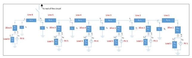
Figure 3.21. Single-line diagram of the circuit section used for the transient overvoltage study
