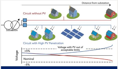
**Figure 1:** An illustration of the increased voltage range in systems with high PV penetration. On a circuit with no PV present (red line), the voltage along the feeder decreases as distance from the substation increases. If the PV power injected into the circuit (blue line) is high enough, the voltage will increase, potentially raising the voltage above normal operational conditions.
