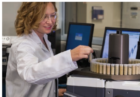
An NREL scientist analyzes herbaceous feedstocks using a near-infrared spectrometer with an autosampler in NREL's Biomass Analysis Technology Lab.
