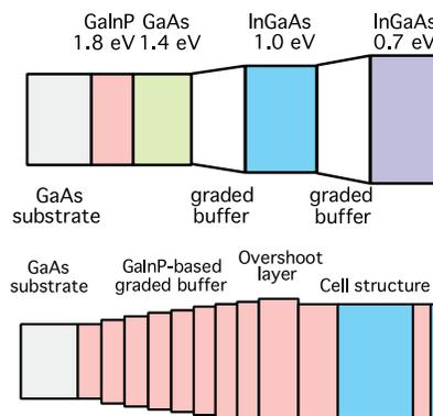
Top: Four-junction inverted metamorphic multijunction structure; profile indicates variations in lattice constants between subcells. Bottom: General structure of compositionally graded buffer and lattice-mismatched solar cell. Illustrations are not to scale. Illustration by Ryan France, NREL
