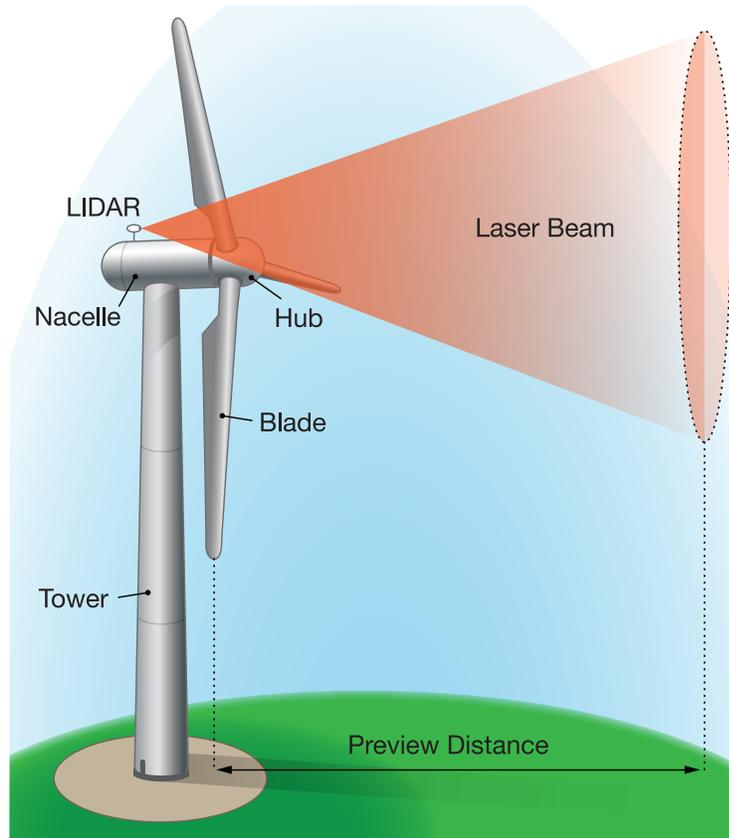
Using laser technology known as a light detection and ranging system, or lidar, NWTC researchers can provide a look-ahead capability. The lidar allows the turbine to effectively “brace itself” for a wind gust before that gust actually arrives, measuring wind speed approximately 50 to 100 meters ahead of the turbine. *Illustration by Al Hicks, NREL*
