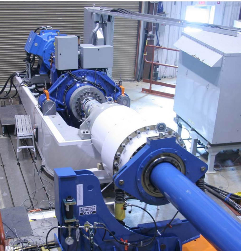
A GRC test article in the NWTC's 2.5-megawatt dynamometer. Photo by Scott Lambert, NREL 19222
