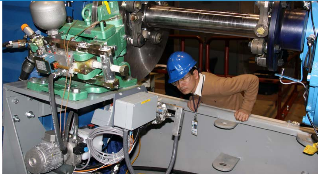
An NWTC engineer inspects the monitoring system for a GRC study. Photo by Joe Verrengia, NREL 16867
