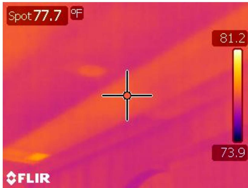
Figure 30. Infrared image of attic duct chase during heating operation
