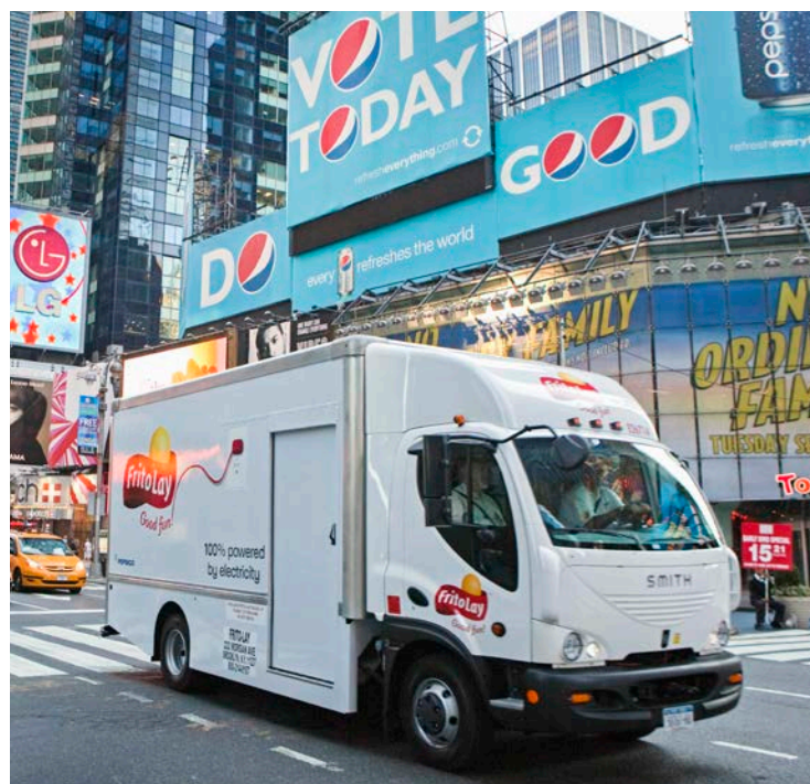
This all-electric vehicle operates at peak effectiveness in urban applications that demand heavy "stop-and-go" driving. Photo from Smith Electric Vehicles, NREL 22851
